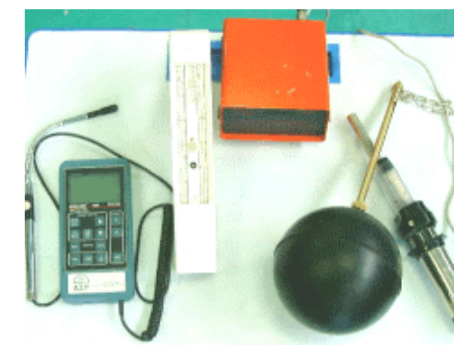
Thermometre, hygrometre, black globe, anemometre used to obtain the thermal index *Wet Bulb Globe Temperature (WBGT)
